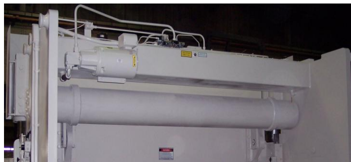
Bushings and bearings are included in the heavy seamless torque tube. The torque tube linkage includes split links and, zero clearance, Teflon bearings.
