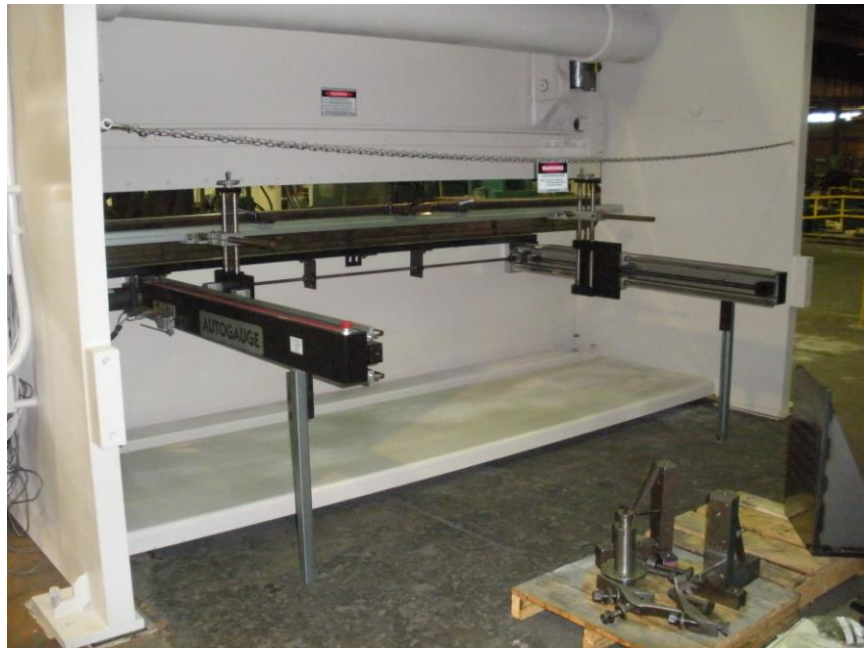
Automec, 48" range X-axis back gauge is controlled through the Automec CNC300 control. Ram depth is also controlled through the Automec.
